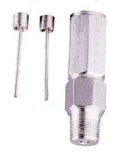
Each snubber is supplied with pistons of three different diameters. Depending on viscosity of the fluid and amount of dampening desired, piston size should be selected. Each piston is marked with numbers 1,2 and 3. Piston 1 should be used with fluid having less viscosity or where higher dampening is required. Piston 3 should be used where fluid viscosity is more or where less dampening is preferred.
